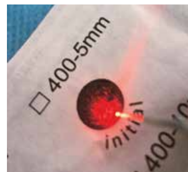
4.30 Incorrect fiber cutting, with obvious irregularities of the laser beam.
