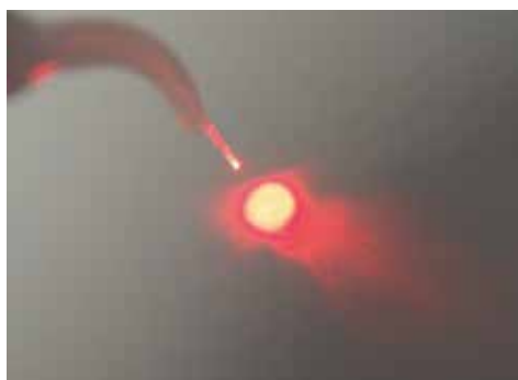
4.28 Properly performed fiber cutting results in a regular laser emission area.
