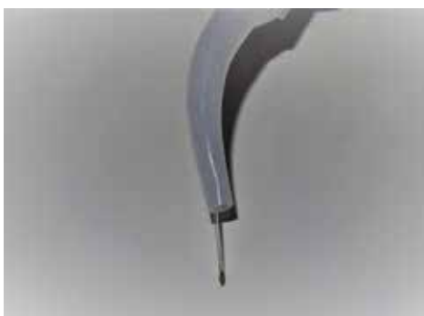
4.32 Activated optical fiber, which can be defined by the blackening of its terminal point.
