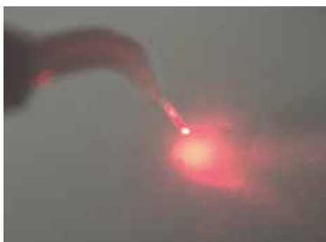
4.29 Incorrect fiber cutting, with obvious irregularities of the laser beam.
