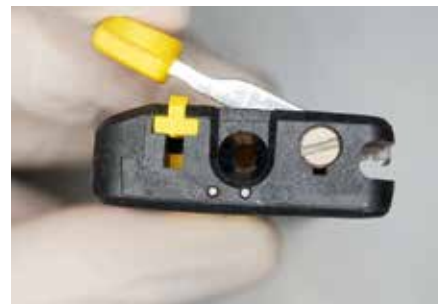
📷 4.27 Special inputs for the optical fiber that allow it to be cut (to the right of the instrument) and the removal of the sheath (in the center of the instrument).
